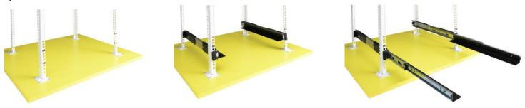
**3.2.** Place the ARAD enclosure onto the slid-out ARAS rails. Next, bolt it from the inside with M4 screws (included). The enclosure is to be fixed to the front part of the RACK rails with four 4xM6 screws.
