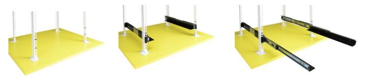
**3.2.** Place the ARAD enclosure onto the slid-out ARAS rails. Next, bolt it from the inside with 4xM4 screws (included). The enclosure is to be fixed to the front part of the RACK rails with four M6 screws.
